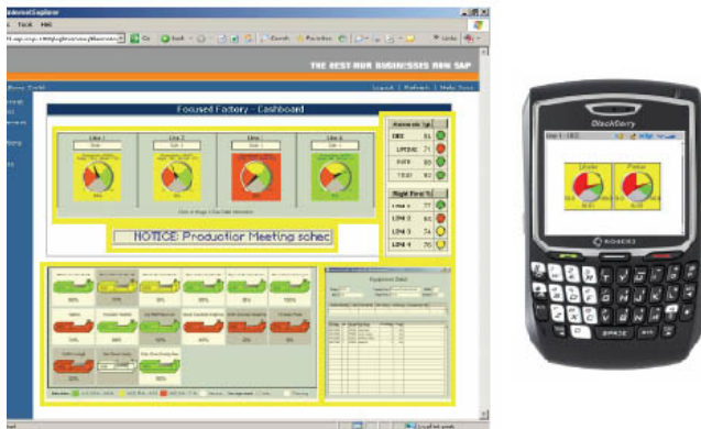
Caption: Using web-based dashboards, key performance indicators (KPIs) can be presented in a role-based and target group specific manner (Source: Siemens IT Solutions and Services 2009)
